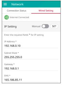
When the [Connection Type] option in the [Connection Status] is set to [Wired]. Wired connection options are displayed.
