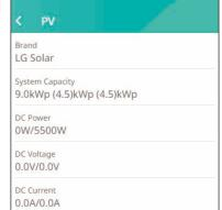
Displays the generating status of the connected PV briefly. The status values are the sum of PV1 and PV2.
