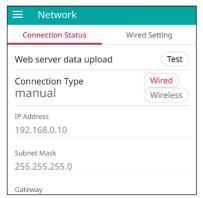
Select [Network] in [Installer Settings]. The current status of the network connection is displayed.
