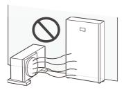
When installing the product next to an outdoor air conditioning unit, install the product in a position that avoids any hot air expelled from the air conditioning unit.
