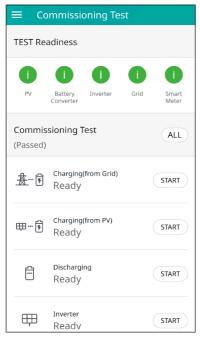
Tab [Operating Test] on [Installer Settings]. The operating test menu is displayed.
