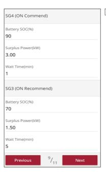
2 DIGITAL INPUT (SG Ready): There are SG4 (ON Commend), SC3 (ON Recommended), and Normal; additionally, Battery SoC, Surplus Power, and Wait Time can be set.
