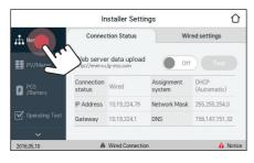
Tab [NETWORK] on [Installer Settings]. Current status of the network connection is displayed.
