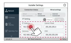
Fill in [PMS IP address], [Subnetmask], [Basic gateway] and [DNS address] option manually.
