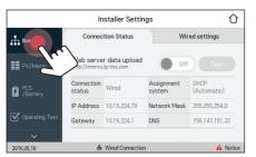
Tab [NETWORK] on [Installer Settings]. Current status of the network connection is displayed.
