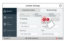
Tab [Wired Settings]. Wired connection options are displayed. If [IP Setting] option in [Wired Settings] tab is set to [Auto], this product will be automatically allocated an IP address from local area network (LAN) via wired connection. You may need to set network connection manually depending on the network conditions. In this case, tab [Auto] to change to [Manual].
