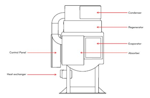
Figure 1-9 Rear view of main body
