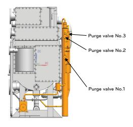
Figure 3-11. The structure of the purge unit
