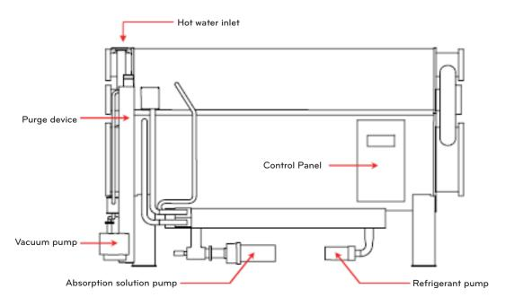
Figure 1-10 Side view of main body (high temp. regenerator side)
