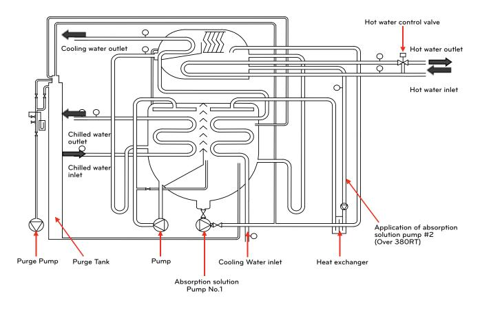
Figure 1-17. Layout of hot water type absorption chiller
