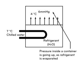
Figure 1-1. Cooling principle (evaporator)
