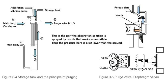
① Absorption solution flows from absorption solution pump to header of storage tank.
