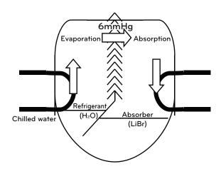
Figure 1-2. Evaporator and Absorber
