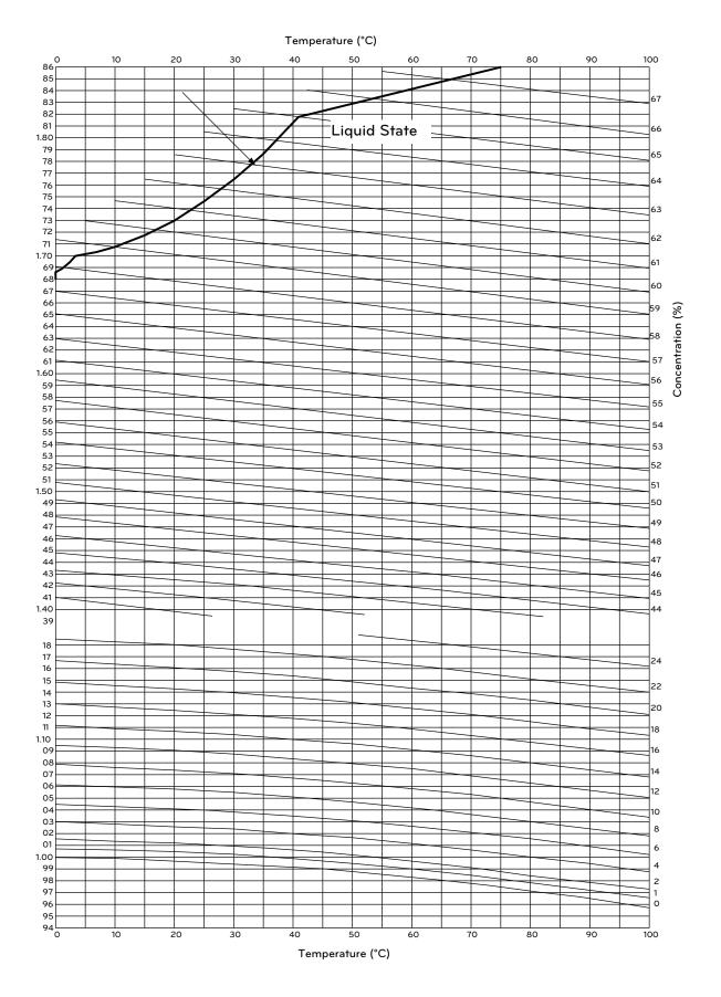
Figure 1-7. concentration curve of absorption solution
