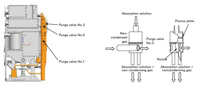
Figure 3-3 Structure of purge unit
