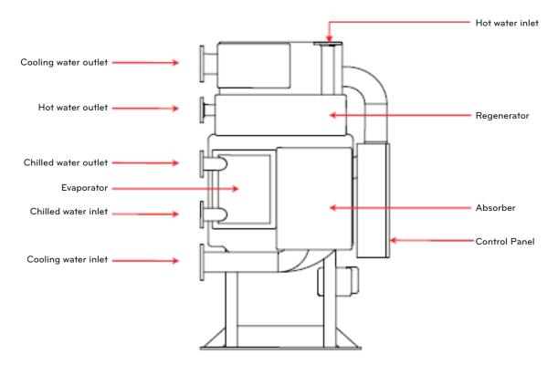
Figure 1-8 Front view of main body
