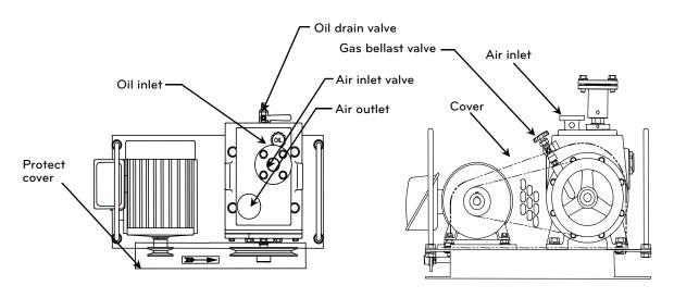
Figure 3-2 Name of purge pump parts
