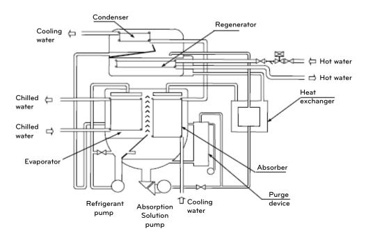
Figure 1-4. Basic cycle of absorption chiller
