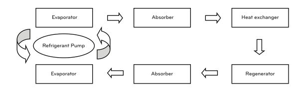
Figure 1-18. The circulation cycle of the absorption solution and refrigerant
