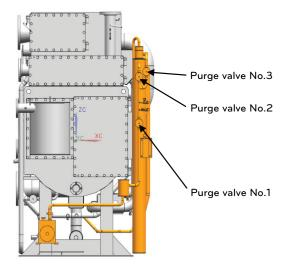
Figure 3-10 Structure of purge unit
