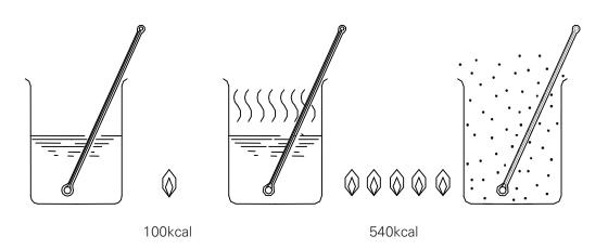
As shown above, using heat of vaporization rather than sensible heat, generated from 1kg (1 $\ell$ ) water, can transfer much more heat capacity. And water is normally evaporated at 100°C. But it can be evaporated at a lower temperature when air pressure is lowered. It is the reason why rice is half-cooked on a high mountain.
