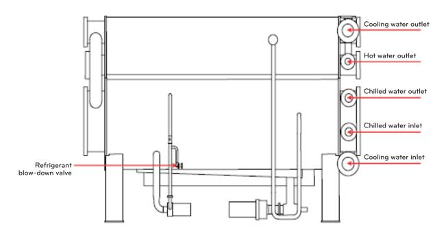
Figure 1-11 Side view of main body (Evaporator side)
