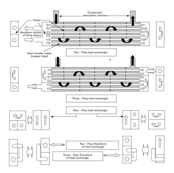
Figure1-16. Heat exchanger
