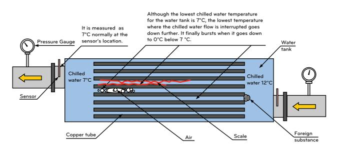
Figure 5-3. The cause of copper tube burst
