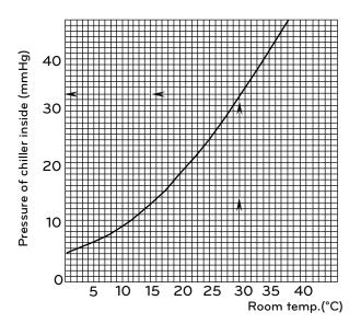
Figure 3-9. Permitted vacuum pressure curve
