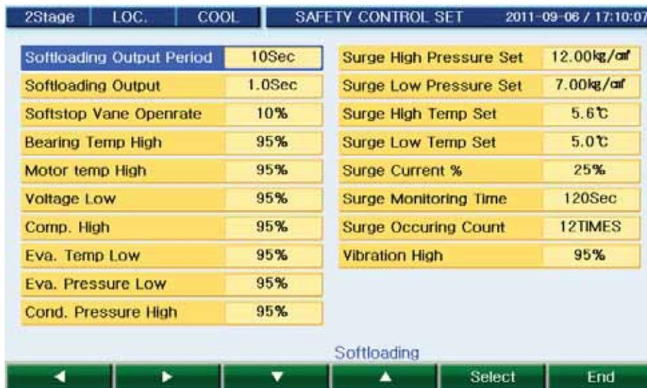
Fig 41. Safety control setting screen
