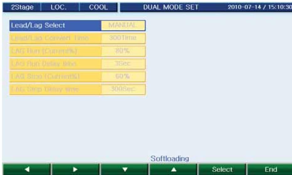
Fig 31. Dual operation setting screen
