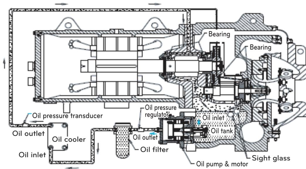
Figure 9. Lubrication cycle
