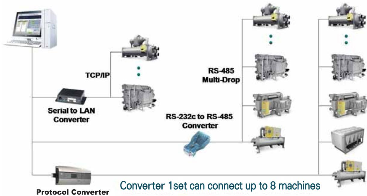
Fig 17. Detail diagram of BMS
