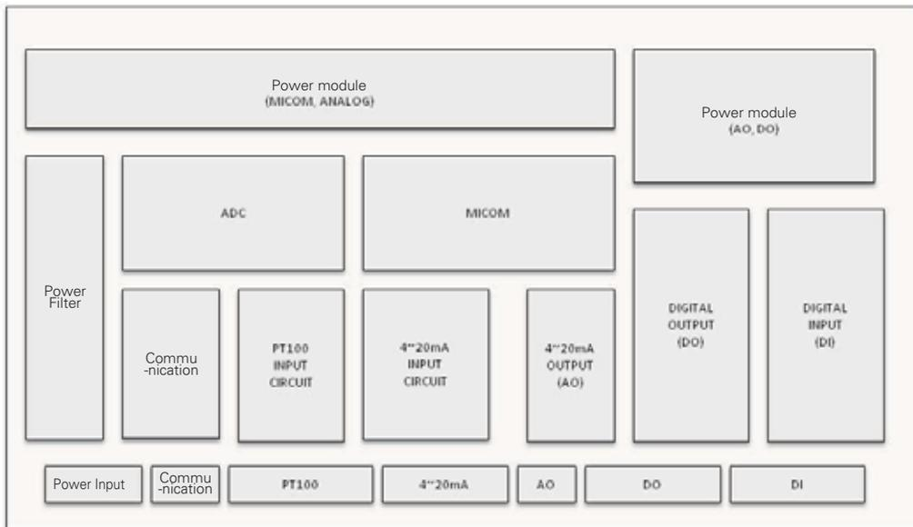
Figure 11. Internal diagram of master/slave board
