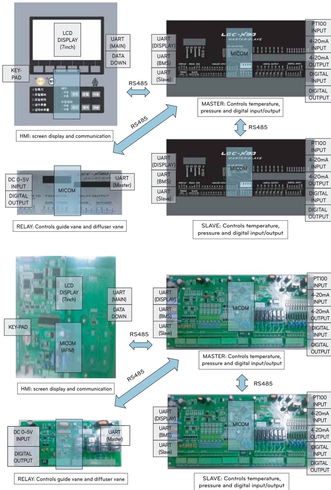
Fig 12. Controller block diagram
