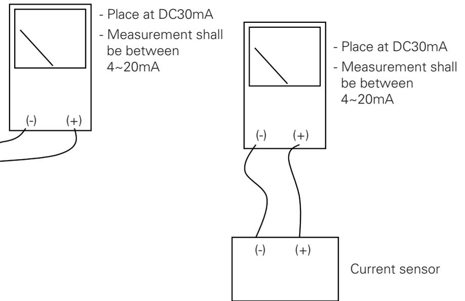
Figure 77. Current sensor measurement circuit
