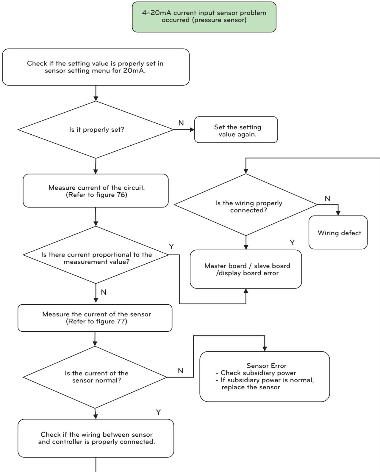
Figure 73. Pressure sensor
