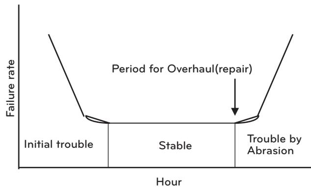
Figure 63. Machine failure rate
