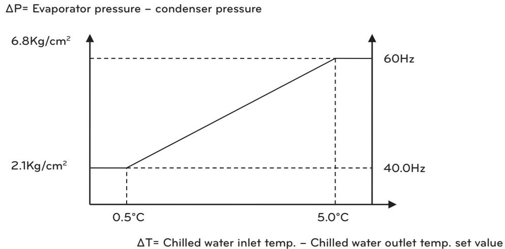
Figure 44. VFD control detail diagram
