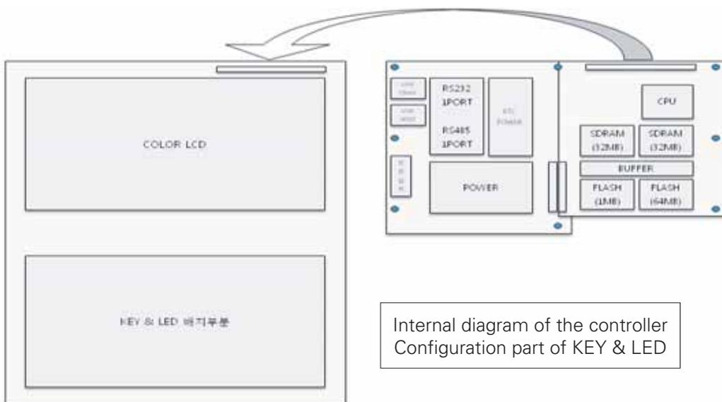
Internal diagram of the controller Configuration part of KEY & LED
