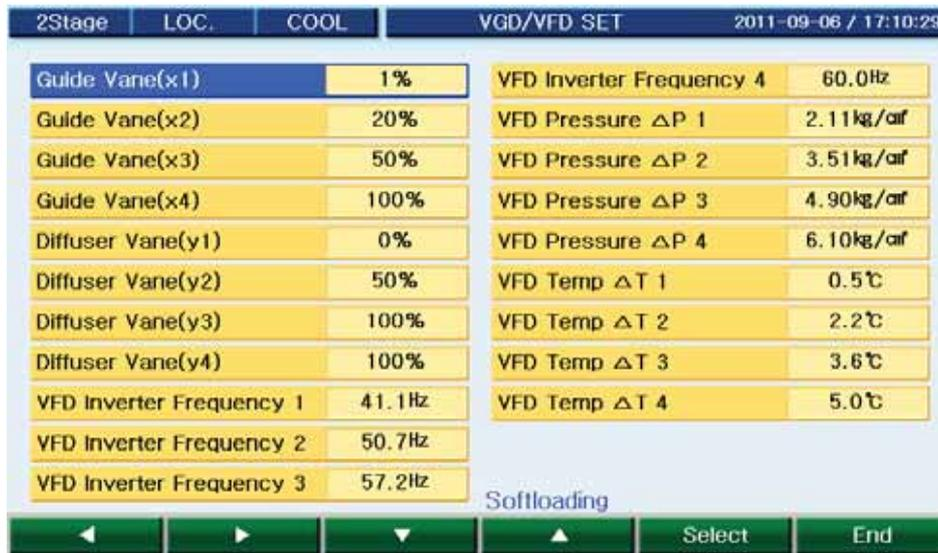
Figure 43. VGD/VFD setting screen
