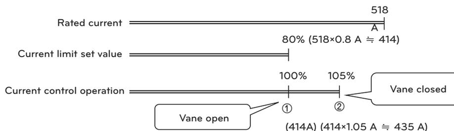
Fig 29. Current limit detail diagram
