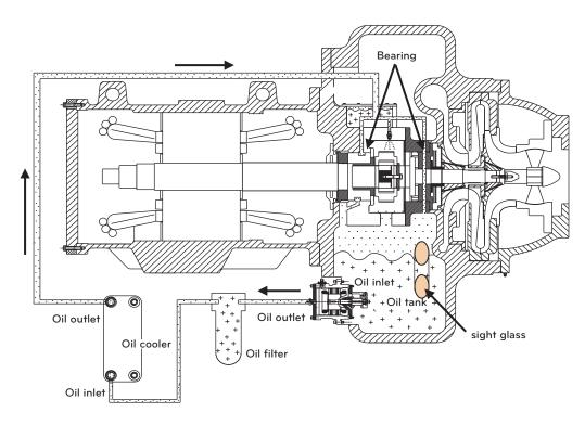
Figure 9. Lubrication cycle
