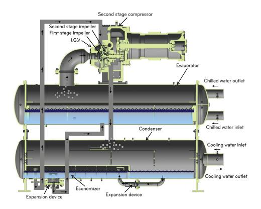
Figure 4. 2-Stage Centrifugal Chiller
