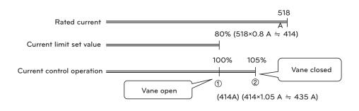
Figure 29. Detailed diagram of current limit
