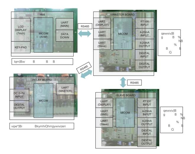
Figure 12. Controller block diagram
