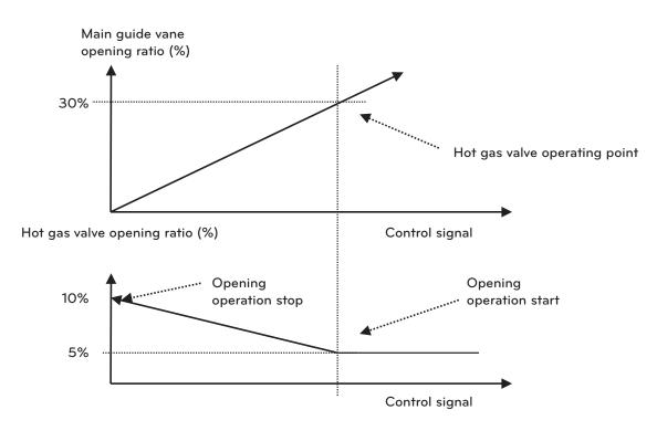
Figure 30. Hot gas valve application diagram
