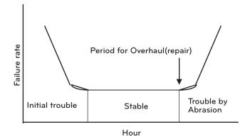
Figure 62. Machine Failure Rate
