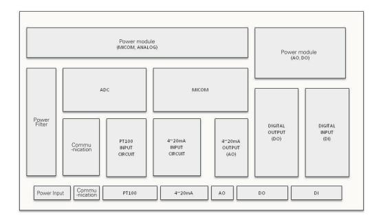
Figure 11. Internal construction of Master/Slave board
