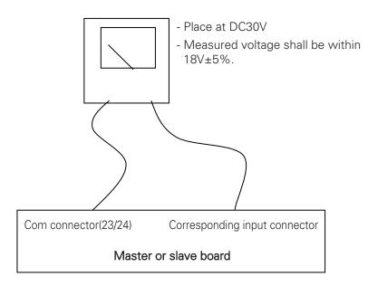
Figure 79. Master or Slave Board Current Measurement Circuit
