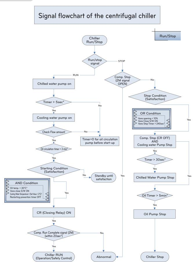
Figure 55. Signal Flowchart
