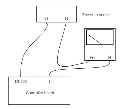
Figure 73. Current Loop Measurement Circuit
