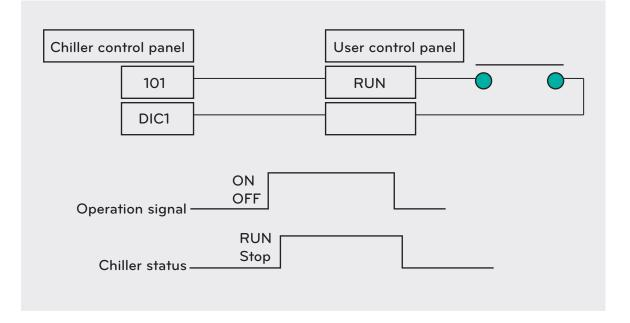
Figure 54. Detailed diagram of remote control signal
