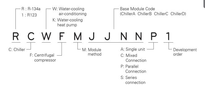
Figure 2. Naming Convention of a Model
