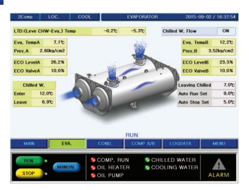
Figure 21. Screen of evaporator
