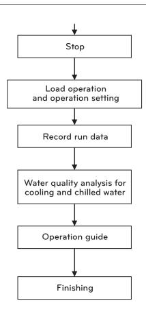
Figure 57. Process from bring-in to test run
