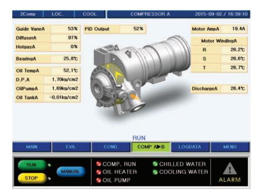
Figure 23. Screen of compressor
