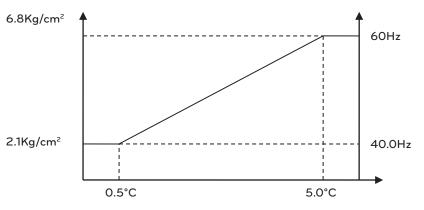
$\Delta T$ = Chilled water inlet temp. – Chilled water outlet temp. set value
