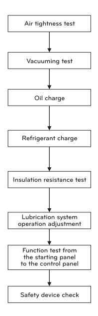
Figure 58. Preparation process for test run
