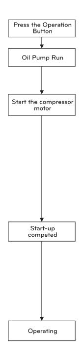
Figure 60. Test run procedure (2)
