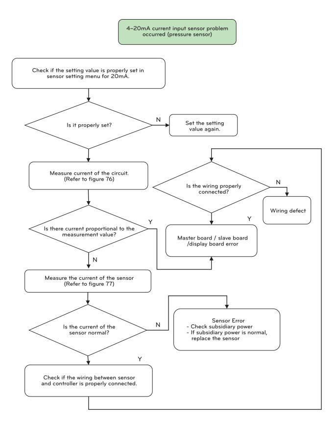
Figure 72. Pressure Sensor
