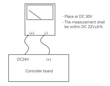
Figure 74. Controller Voltage Measurement Circuit
