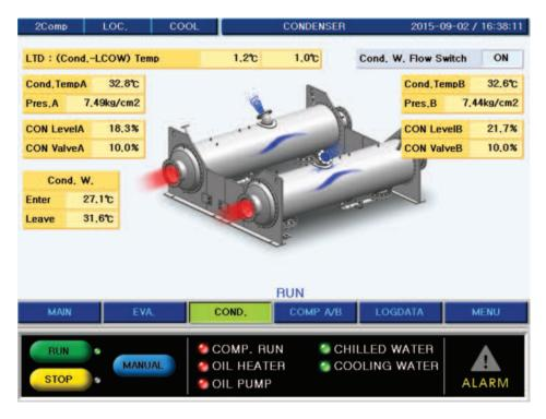
Figure 22. Screen of condenser
