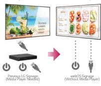
Embedded System-on-Chip (SoC) eliminates the need for external media player and related cable.
