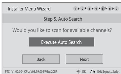
6. Select **Execute Auto Search** (Auto Tuning) and press **OK (Enter)** to start the channel scan (searches for all available analog and digital channels). The system will display progress of the channel scan in a pop-up window.
