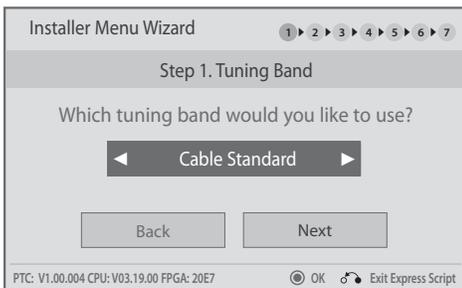
2. Use the Left/Right arrow keys to select the appropriate tuning band (Cable Standard [default], Cable HRC, Cable IRC, or Air). When you have made your selection, use the arrow keys to select **Next**, and then press **OK (Enter)**.
