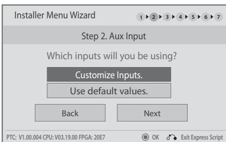
3. Use the Up/Down arrow keys to select the desired Aux input option. (Note: If you simply select **Next** and press **OK (Enter)** in this step, default values will be used.)
