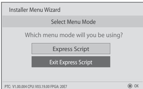
1. Upon launching, the Installer Menu Wizard prompts you to select a preferred Menu Mode. Use the Up/Down arrow keys on the Installer Remote to select/highlight **Express Script** in order to proceed with the Installer Menu Wizard. Then, press **OK (Enter)** on the Installer Remote.
