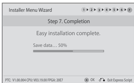
For the final step, the system will save your settings and transfer the setup to the internal TV controller (PTC) (similar to 2-5-5 + MENU Mode). When this step is complete, the system exits the Installer Menu Wizard.
