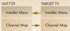
figure 2. DATA FLOW-BETWEEN LMT7Z9 AND TARGET TV Conditions of LMT7Z9: FTG mode previously used in a TV of the same model.
