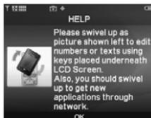
Your VX9400 phone has a swivel LCD. This versatile design allows you to use certain device features while the LCD is down, then swivel the LCD up to the landscape position to reveal the phone's numeric keypad for full use of the phone's functions and features.
