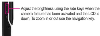
Adjust the brightness using the side keys when the camera feature has been activated and the LCD is down. To zoom in or out use the navigation key.
