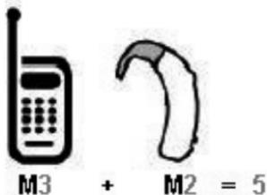
In the above example, if a hearing aid meets the M2 level rating and the wireless phone meets the M3 level rating, the sum of the two values equal M5. This should provide the hearing aid user with “normal usage” while using their hearing aid with the particular wireless phone. “Normal usage” in this context is defined as a signal quality that’s acceptable for normal operation.
