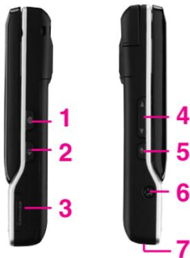
1. **Side Camera Key** Use for quick access to Camera function.
