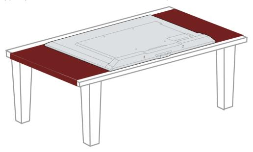
2 Align the TV stands with the screw holes on the bottom of the TV, then secure the stands to the TV with the four provided screws.
