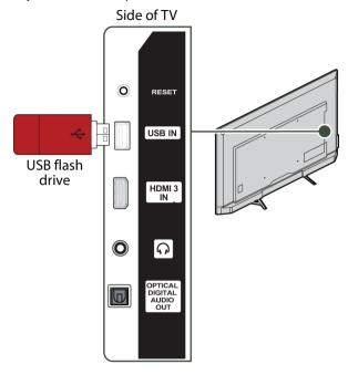
1 Plug a USB flash drive into the **USB IN** port on the side of your TV.
