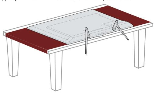
2 If the TV stands are installed, remove the four screws that secure the stands to your TV.
