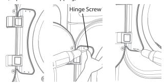
3. Insert latch to right side and install screws.
