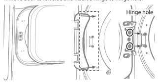
2. Hold on hinge while screw down a hinge (to prevent door dropping).
