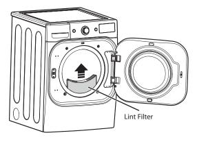
To clean, open the dryer door and pull the lint filter straight up.
