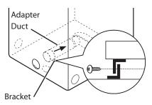
3. Insert the 4 inches (10.2 cm) elbow through the rear opening and press it onto the adapter duct. Be sure that the male end of the elbow faces down through hole in the bottom of the dryer. Secure in place with duct tape.
