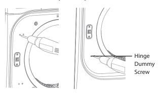
4. Remove two screws and disassembly Latch.
