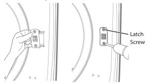
4. Screw down four dummy screws right side.
