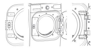
3. Remove four dummy screws by driver.
