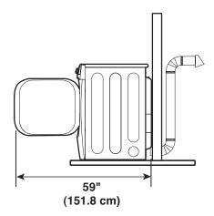
If the duct isn't installed in the wall.
