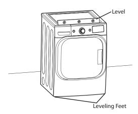
All four leveling feet must rest solidly on the floor. Gently push on the top corners of the dryer to make sure that the dryer does not rock from corner to corner.
