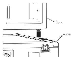
4. Insert the front rail between the bottom of the dryer and the top of the washer. Push the front rail toward the back of the washer until it comes in contact with the side rail stoppers. Install the two remaining screws to secure the front rail to the side rails.
