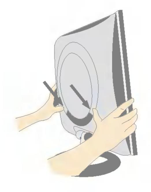
**4.** Insert the back cap along the bottom grooves on both sides, holding the bottom.
