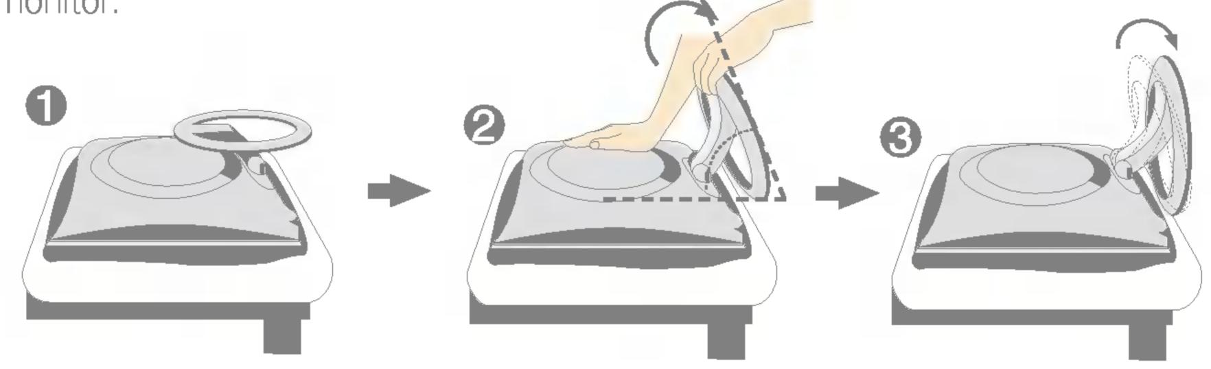
**4.** Place the monitor upright and adjust the stand base angle as desired. Adjust the stand base angle holding the monitor head part with both hands.
