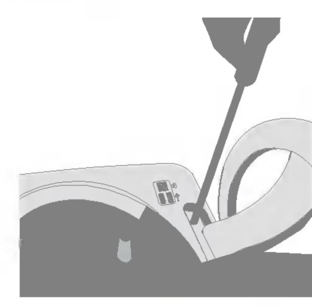
3. Separate the stand base using a screwdriver as shown in the picture.
