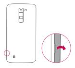
Rasics 18 2 Slide the Nano SIM card into the Nano SIM card slot as shown in the figure. Make sure the gold contact area on the card is facing downward.
