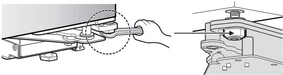
\* It is convenient to use the small hole on the back of the spanner included in the accessory box.
