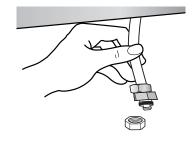
Prepare a bucket under the water service pipe connector before checking for any water leakage to avoid ruining the flooring material and carpet etc.
