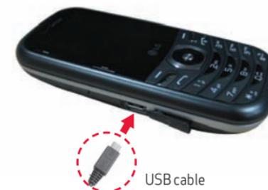
NOTICE: Please make sure that the "B" side faces up before inserting a charger or USB cable into the Accessory/Charger Port of your phone.
