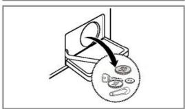
**3.** Remove out any foreign material from the pump filter (③).
