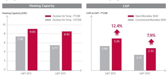
1) Normal : Outdoor air temperature 7°CDB / 6°CWB, Water outlet temperature 35°C
