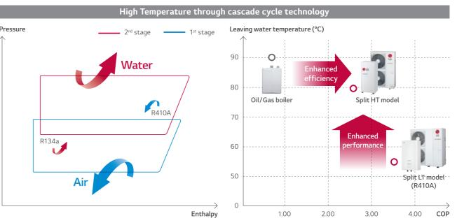
$^{\star}$  Condition for HT model: outdoor air temp. 18 °C, entering water temp. 70 °C \* Condition for LT model: outdoor air temp. 18°C, entering water temp. 55°C
