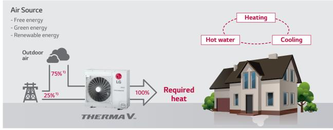
1) This is a general ratio based on LG Therma V R32 Series vs. electrical boiler under low temperature & average climate conditions, which may differ from actual operation.
