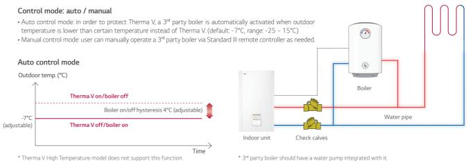
$<sup>^{\</sup>star}$  3<sup>rd</sup> party boiler should have a water pump integrated with it.
