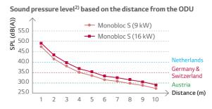
1) Minimum distance to be away from a neighboring property may vary depending on installation conditions and noise regulations in individual countries. 2) Sound pressure level is converted from sound power level of low noise mode based on a tonality penalty of 0 dB and installation in free-field. The directivity index (Q) is assumed as 2.
