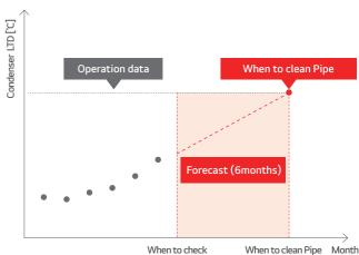
→ Condenser heat exchanger needs inspection after 6 months of customs.
