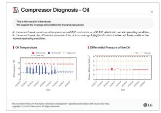
By using oil differential pressure, you can know in advance when to change the oil filter.
