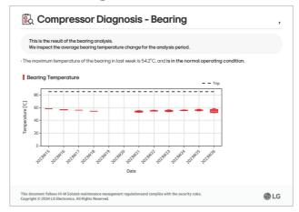
Oil and bearing temperature monitoring prevents compressor burnout.
