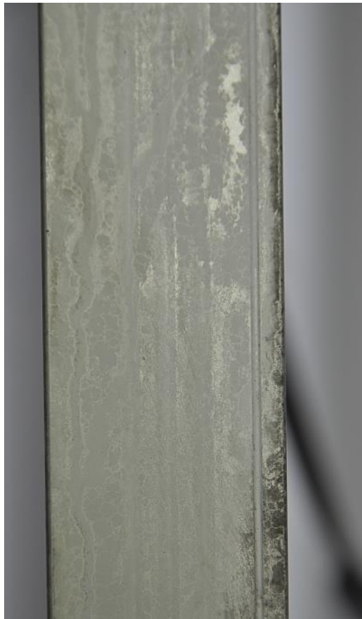
Fig. 6: detailed side view to frame after ammonia corrosion test
