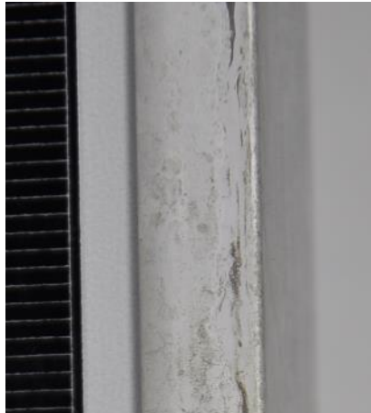
Fig. 6: detailed side view to frame after ammonia corrosion test
