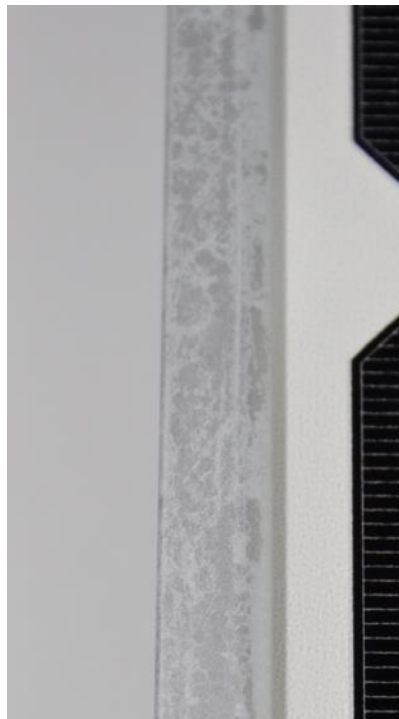
Fig. 6: detailed left side view to frame after ammonia corrosion test
