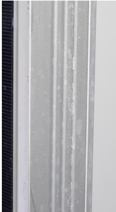
Fig. 6: detailed left side view to frame after ammonia corrosion test
