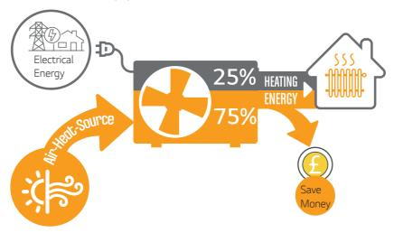
Image above: Example diagram 'How an air-to-water heat pump works'.
