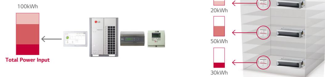
※ Outdoor unit's accumulated electric energy / using rate of individual indoor unit + indoor unit's accumulated electric energy is displayed in wired remote controller, only when central controller, digital integrating electricity meter and PDI are installed and PDI, outdoor unit and indoor unit are connected with power wire. Only total accumulated electric energy is displayed in standard wired remote controller. In premium wired remote controller, that are displayed into week / month / year.
