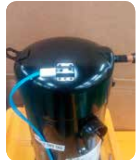
4 Slide out the protector, slide in replacement, and reinstall the cover
