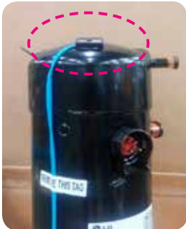
1 Locate top cap and thermal protector on the dome
