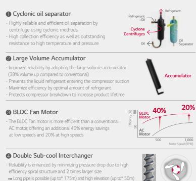
$\rightarrow$  Reduction of indoor refrigerant noise level \* Based on equivalent pipe length
