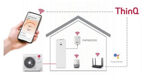
PWFMDD200 (LG Wi-Fi modem) / PWYREW000 (10 m extension connect cable in between Therma V indoor and LG Wi-Fi modem) could be required depending on installation conditions
