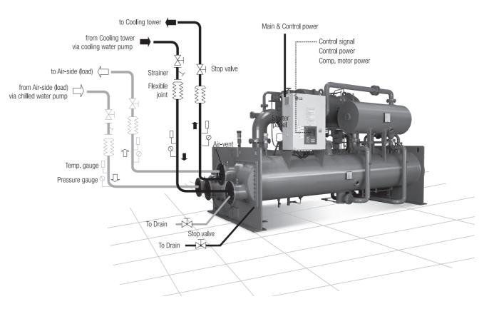
Notes: 1. Control power - 3Phase/220V/50Hz(60Hz) - should be provided by the customer apart from main power source. 2. The Main power wiring to the starter and 2nd wiring between the chiller and starter must be done based on local regulation. And the work scope is purchaser's.
