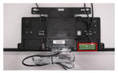
Remove the power cord bracket and power cord.
