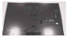
Remove screws to remove the back cover and the bottom cover (Tool set up : Screw driver with "+" tip.)
