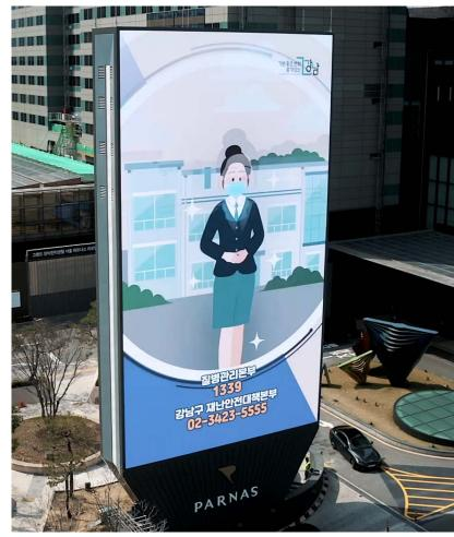
LG's eye-catching LED Signage solution is hard to miss. Two strikingly vibrant 10,000 nit displays – 71.5 feet tall by 39.3 feet wide – are embedded in a structure that measures an imposing 85.3 feet in height.
