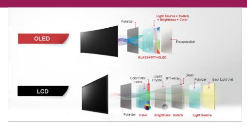
OLED-based displays are self-lighting displays without BLU liquid crystal. The viewer sees each pixel directly because the color saturation, contrast, and off-axis viewing are far superior to images on LCD panels.
