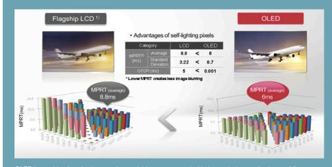
OLED is capable of a refresh rate as low as 0.001ms, compared with the much slower refresh rate of 5ms for LCD. OLED processes and changes content 5,000 times faster than a standard LED-backlit LCD panel. Additionally the lower Motion-Picture Response-Time metric (MPRT) (i.e., the time it takes for a pixel to go from black to white to black again) means less image blurring with OLED versus LCD.
