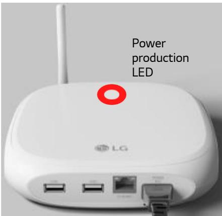
At least one Micro Inverter does not produce power over 72 hours
