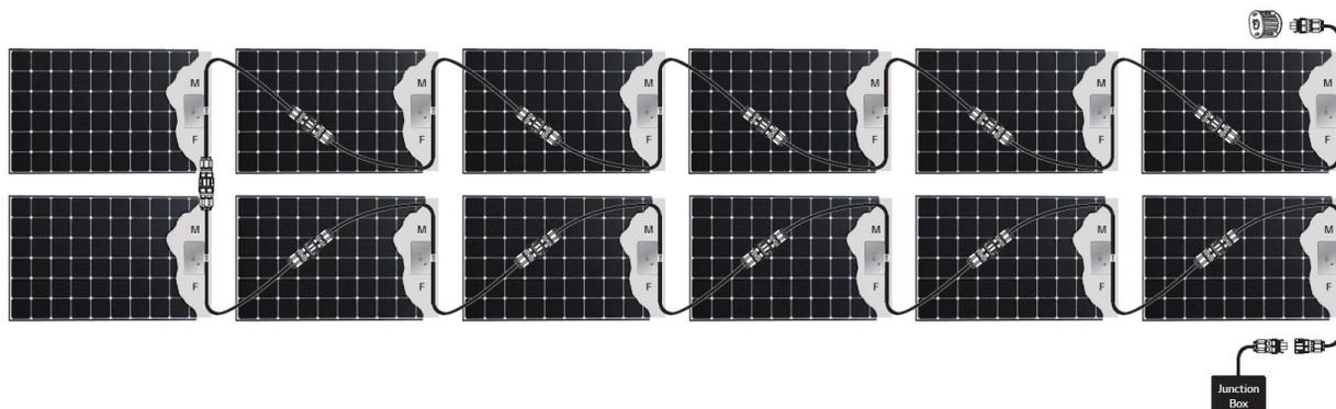
If AC junction box is on the left side of a 2-by-6 PV array in landscape orientation,
