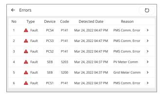
[Type] shows the severity of the error, [Device] shows the information of the device where the error occurred, and [Code] shows the error code.
