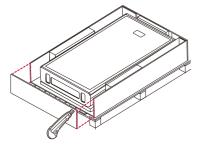
Cut the bottom of the package.
