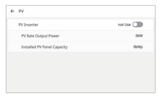
If you are using a PV inverter, set the [PV Inverter] option to [Use] and fill the [PV Rate Output Power] and [Installed PV Panel Capacity] fields.
