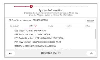
When next step button is pressed, If the ESS information detected at the initial booting is different from the current information, reboot and refresh the initial information.
