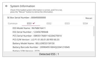
When back button is pressed, If the ESS information detected at the initial booting is different from the current information, reboot and refresh the initial information.
