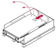
Move the Home 5/8 to stand on the bottom side by lifting the top of the product while the Home 5/8 Legs are out of the pallet, then stand the Home 5/8 upright.
