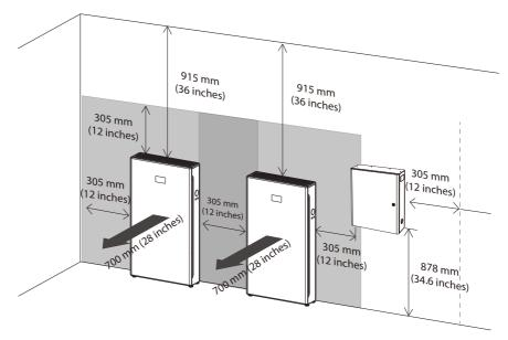
This product must be installed with clearance at the left, right, top, bottom and front of the product as shown in the figure.
