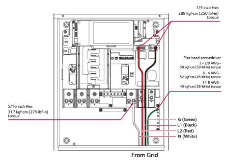
2 Connect the home load conductors (L1, L2, Neutral, and Ground) to the SE Box backup load terminals as in the following figure.
