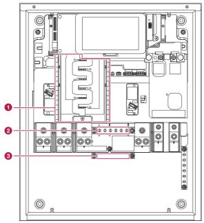
The internal Panelboard is 200A-rated and supports  $5 \times 2$ -pole breaker spaces (10 circuits) using Eaton BR Branch circuit breakers up to 125 A.
