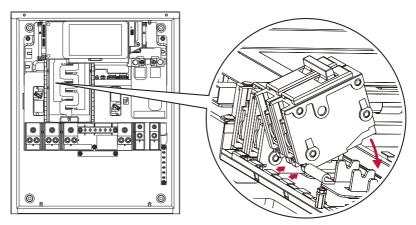
Pass the PV L1 cable from the PV inverter through the 200 A CT as shown below. The side with 2 the markings P1 and K on the CT faces the PV inverter, and the side with the L and P2 faces the SE Вох.
