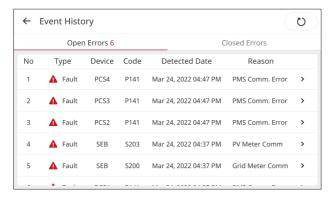
[Level] shows the severity of the error, [Device] shows the information of the device where the error occurred, and [Code] shows the error code.
