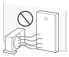
When installing the Home 5/8 next to an air conditioner outdoor unit, install the Home 5/8 in a position that avoids any hot air expelled from the air conditioner outdoor unit.
