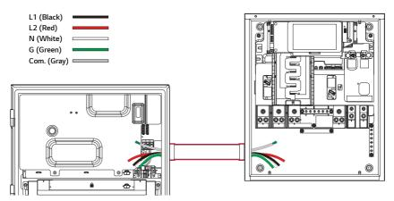
Strip off the AC power conductors (L1, L2, Neutral, and Ground) on both the Home 5/8 and SE Box sides as shown in the figure below.
