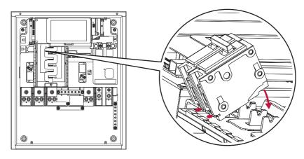
On the SE Box side, connect the AC conductors to the corresponding terminals as shown in the figure.
