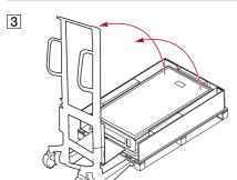
Put the hand lift into the bottom of the package and stand the Home 5/8 upright on the hand lift.
