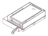
Cut the bottom of the box so that the hand lift can fit through the bottom.
