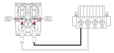
After connecting the end of the CT Harness to pins 1 and 2 of the terminal block for PV CT in the SE Box, respectively, S1 (PV L1+) and S2 (PV L1-), plug it into the connector and tighten the screws on both sides of the terminal block.
