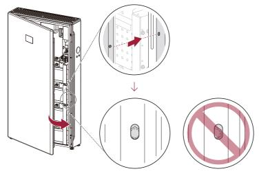
$\fbox{\textbf{7}} \quad \text{Fasten the screws on the right side of the Home 5/8. (25 kgf·cm (22 lbf·in) torque, Hex socket : M8)}$
