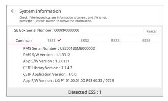
You can check the information of the installed ESS on the system information screen. If Home 8 is connected to SEBox, ESS mode name is displayed "RA768K16A11". If Home 5 is connected, it is displayed "RA500K16A11".
