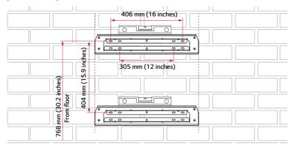
Affix the wall bracket to the wall with screws or anchors.
