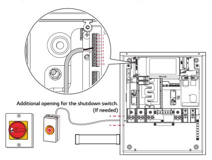
Confirm that all Home 5/8 operation is shut down when the switch is pressed with a plunger type switch or OFF position with the rotary type switch.
