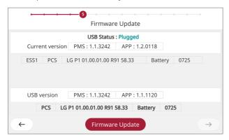
The current version and new version of the system firmware are displayed. Connect a USB storage device containing the latest software to the USB connector and press [Firmware update] to start the firmware update.
