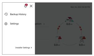
To enter the Installer settings menu, you need to input the password on the screen. Input the password to enter the settings menu.
