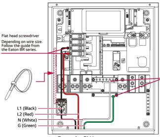
Flat head screwdriver 2 – 2/0 AWG – 58 kgf·cm (50 lbf·in) torque 6 – 4 AWG – 52 kgf·cm (45 lbf·in) torque 14-8 AWG – 40 kgf·cm (35 lbf·in) torque
