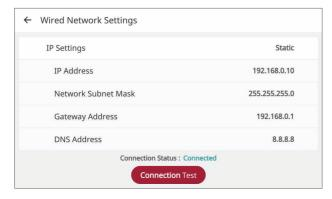
If the [IP Settings] option is set to [DHCP], the system will automatically be allocated an IP address from the local area network (LAN) through the wired connection. You may need to set the network connection manually depending on the network conditions. In this case, press [DHCP] to change to [Static].
