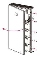
Remove the screws on the right side on the front cover starting from the bottom and working your way up, and then open the front door of the Home 5/8.
