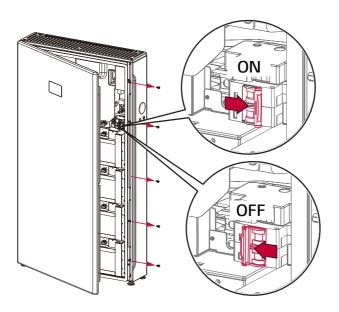
Pass the 6-conductor communication cable and the AC power conductors (L1, L2, Neutral and Ground) through the conduit installed between the Home 5/8 and SE Box.
