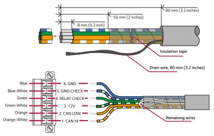
$\cite{7}$  On the SE Box side, strip the 6-conductor communication cable as shown in the figure.
