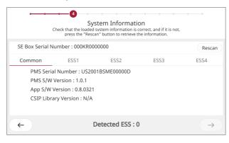
Check that the loaded system information is correct. If it is not, check the DIP switches on each Home 5/8 and press [Rescan] to retrieve the information.
