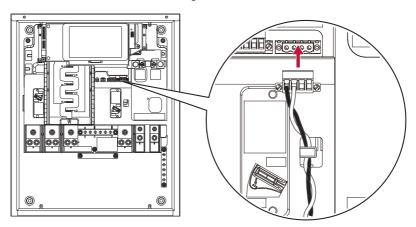
Connect the PV inverter conductors (L1, L2, Neutral, and Ground) to the corresponding terminals as shown in the figure.
