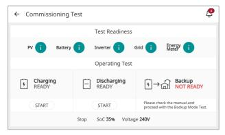
The Charge and Discharge tests are each around 10 minutes. The result is displayed when each test is completed. When there is no problem with the test, [Success] is displayed. When [Fail] is displayed, press each test result to display the detailed information. Check and solve the errors by referring to the error code in the information, then perform the test again. For information on an error code, refer to "Error Codes and Messages".
