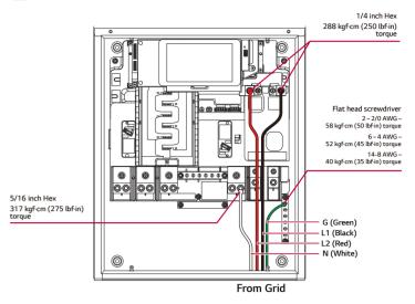
Connect the home load conductors (L1, L2, Neutral, and Ground) to the SE Box backup load terminals
