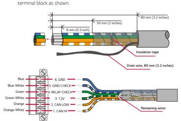
6 On the SE Box side, strip the 6-conductor communication cable as shown
