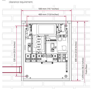
Fix the SE Box with 4EA screws and anchors with O-rings in each position. Before fastening the screws, place the supplied O-rings on the screws.
