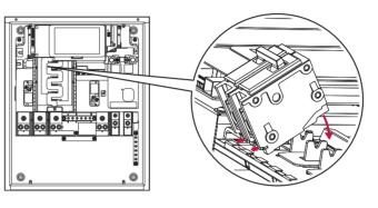
[10] connect the AC conductors to the corresponding terminals
