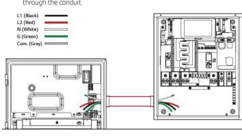
3 Strip off the AC power conductors (L1, L2, Neutral, and Ground) on both the Home 5/8 and SE Box sides as shown in the figure below.
