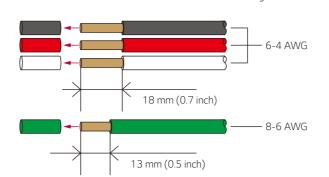
Connect the AC conductors to the corresponding terminals and connect the AC power ground
