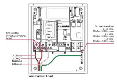
3 Connect the non-backup load conductors (L1, L2, Neutral, and Ground) from the non-backup panel to the SE Box non-backup load terminals
