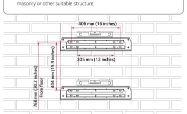
Affix the wall bracket to the wall with screws or anchors.
