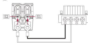
[4] Plug the terminal block into the connector and tighten the screws
