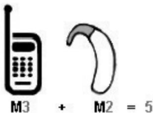
In the above example, if a hearing aid meets the M2 level rating and the wireless phone meets the M3 level rating, the sum of the two values equal M5. This should provide the hearing aid user with “normal usage” while using their hearing aid with the particular wireless phone. “Normal usage” in this context is defined as a signal quality that is acceptable for normal operation.
