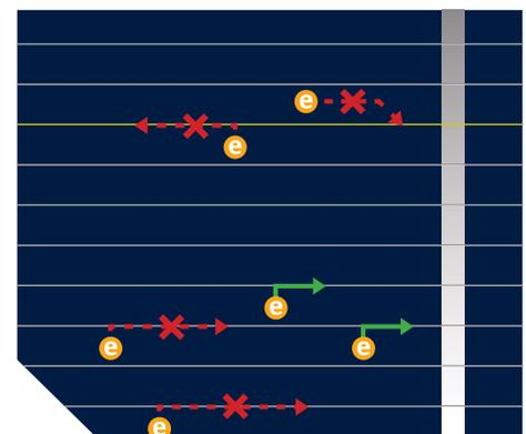
Multiple electrical paths maintained by wires
