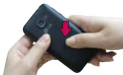
**3** Place the battery cover over the battery compartment, then press it downward until it clicks into place.
