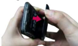
**1** Use the fingertip cutout at the bottom of the phone to remove the back cover.
