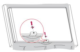
2 After removing the screw, remove the LG Logo Bracket. Align with the hole on the left side to attach the LG Logo Bracket with a screw.
