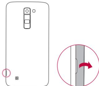
2 Slide the SIM card into the SIM card slot as shown in the figure below.
