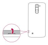
2 Slide the SIM card into the SIM card slot as shown in the figure below. Make sure the gold contact area on the card is facing downward.
