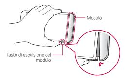
2 Grab the middle of the ejected module and pull it out from the device.
