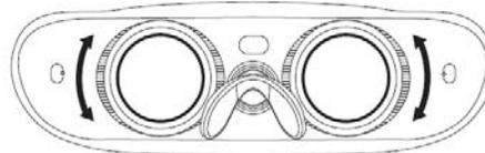
**5** Adjust focus manually by rotating. (360 VR provides optimal viewing and is intended for use without glasses, as the lenses will adjust according to your vision.)
