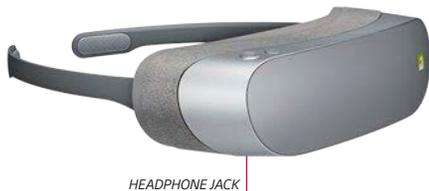
**7** For audio playback during your VR experience, you can either listen directly from the LG G5's speakers, or plug a wired headset into the LG G5 or LG 360 CAM.
