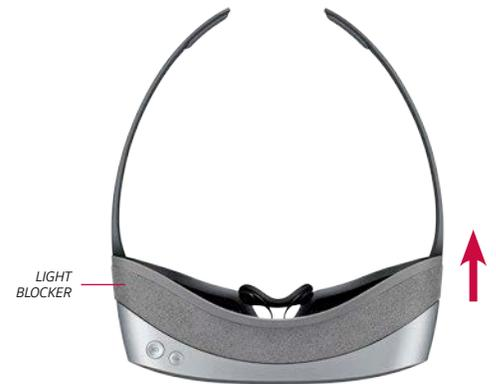
**3** Remove the light blocker and put on the 360 VR. A safety notification will appear – use it as a visual reference to adjust the lenses.
