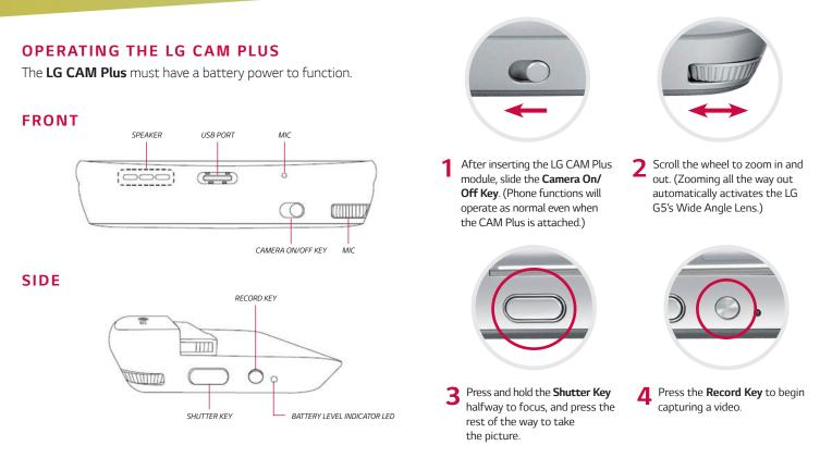
**Notes:** The LG CAM Plus cannot be operated while the USB is connected (data communication and charging are still available). You can only use one LG Friend at a time, OTG devices that are connected to the LG CAM Plus will not be recognized (e.g. LG 360 VR, OTG card readers, etc.).
