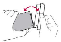
**3** Disconnect the battery from the module by pulling it in an outward arc.
