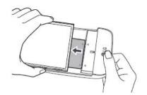
5 Carefully slide the battery and the LG CAM Plus module into the phone until it's closed. You should hear a slight click when it's secured.
