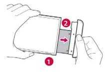
**2** Press the module release button (1) and pull the battery module out to remove it from your phone (2).
