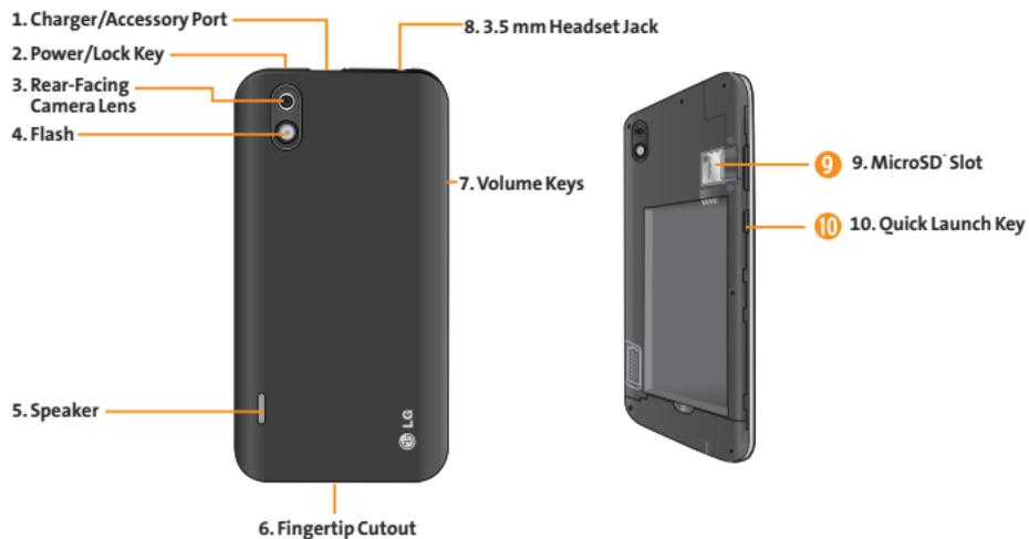
1. **Charger/Accessory Port** allows you to connect the device charger or an optional USB cable. **CAUTION!** Inserting an accessory into the incorrect port may damage the device.
