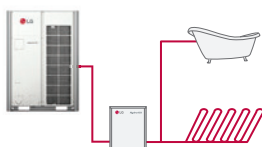
Hot water+ Underfloor heating
